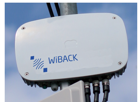
Outdoor WiBACK node (available with 2, 3 and 4 Antennas, see data sheets).
